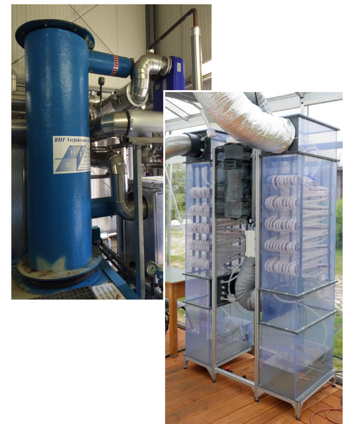
Figure 3: ZHAW and Watergy tested the absorption technology in previous projects: the High Temperature Condensing Technology (ZHAW) in the power plant Berlin Buch, recovers heat from the flue gas in an ab- /desorption process (top); an absorption box of Watergy is installed in a prototype building in Berlin (bottom).
