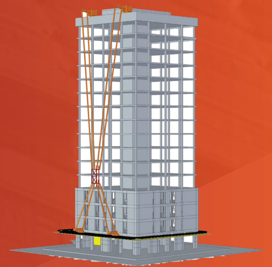
Conceptual view of a cable robot (orange) working on a building. The platform hosting the MEE is coloured red
