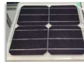
Small prototype with bifacial c-Si cells developed by H2020 BIPVBOOST project (4+4, 360 x 360 mm)
