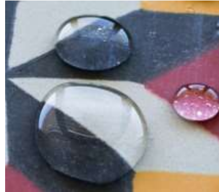
Hydrophobic coating on porous material (TECNAN website)
