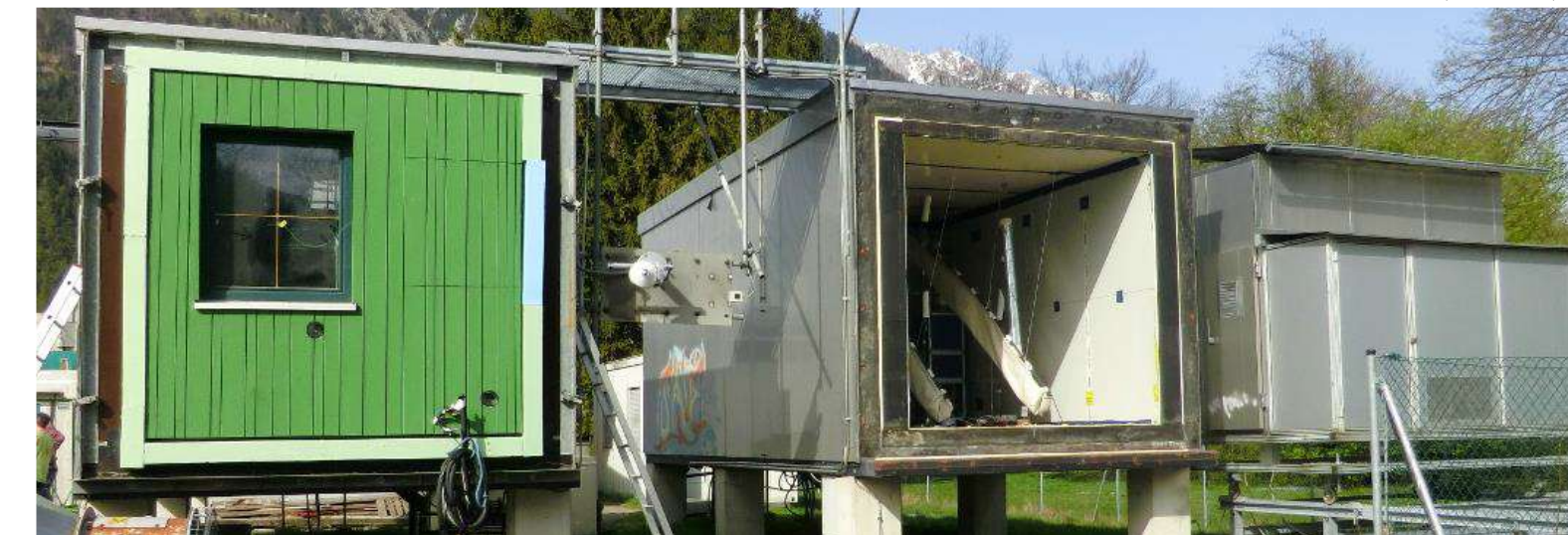
PASSYS outdoor test cells (UIBK)
