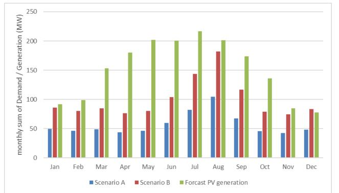
Scenario A: is based on scaling the synthesised demand profile against the measured data.
