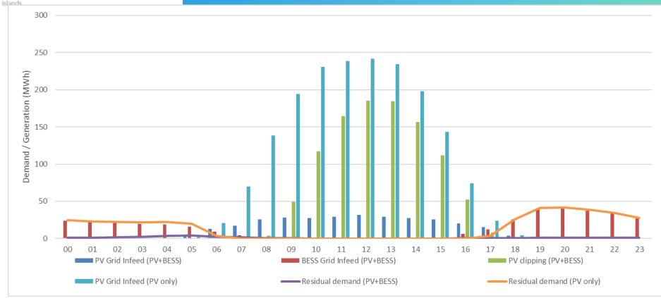
The PV only residual demand (red line) is pronounced throughout the evening peaks and night-time loads: reduced! Morning hours still require some inputs from the grid.
