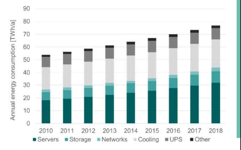
The EU Code of Conduct Data Centres Energy Efficiency identifies data centre cooling (which account for up to 40% of the energy demand) as frequently the largest energy loss in the facility and, as such, represents a significant opportunity to improve the energy efficiency.
