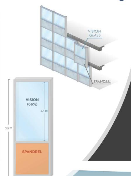
EENSULATE curtain wall modules where the thermal and acoustic insulation are provided by the novel EENSULATE glass based on VIG technology and EENSULATE foam (TCF) in the spandrel combined with SoA low-e coated glass, including thermo-chromic coated glass with additional self-cleaning and antifogging functionalities
