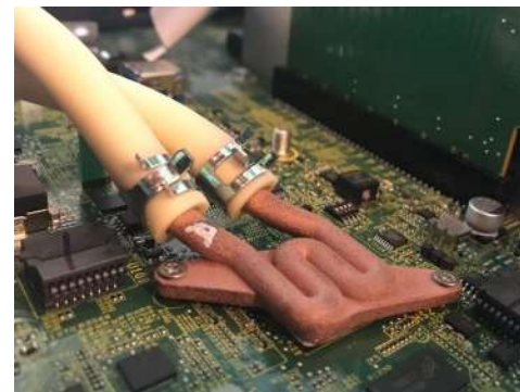
Direct Water Cooling
