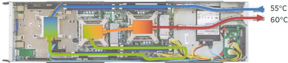
Example: Water-cooled Megware Supercomputing Blade
