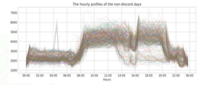
It is possible to visually spot at least three different daily patterns: one where the highload period spans from 09:00 to 19:00, one where the high-load period spans from 09:00 to 13:00, and one that includes an unusual peak during the early morning hours.
