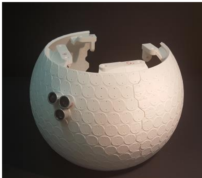
6-pieces rigid 3D printed surfaces with inner structure
