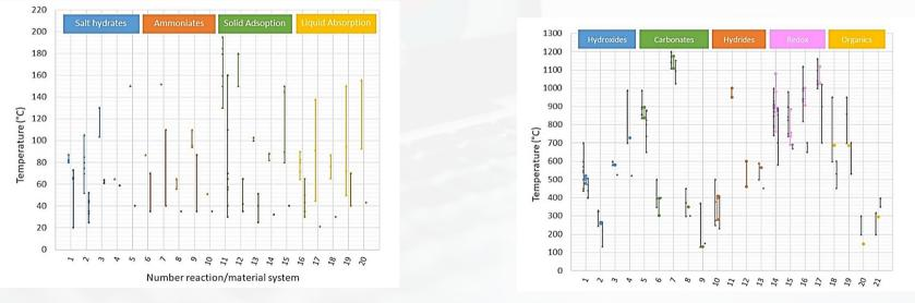
Charge/discharge temperature of selected TcES: left) Low-temperature; right) Medium-High Temperature
