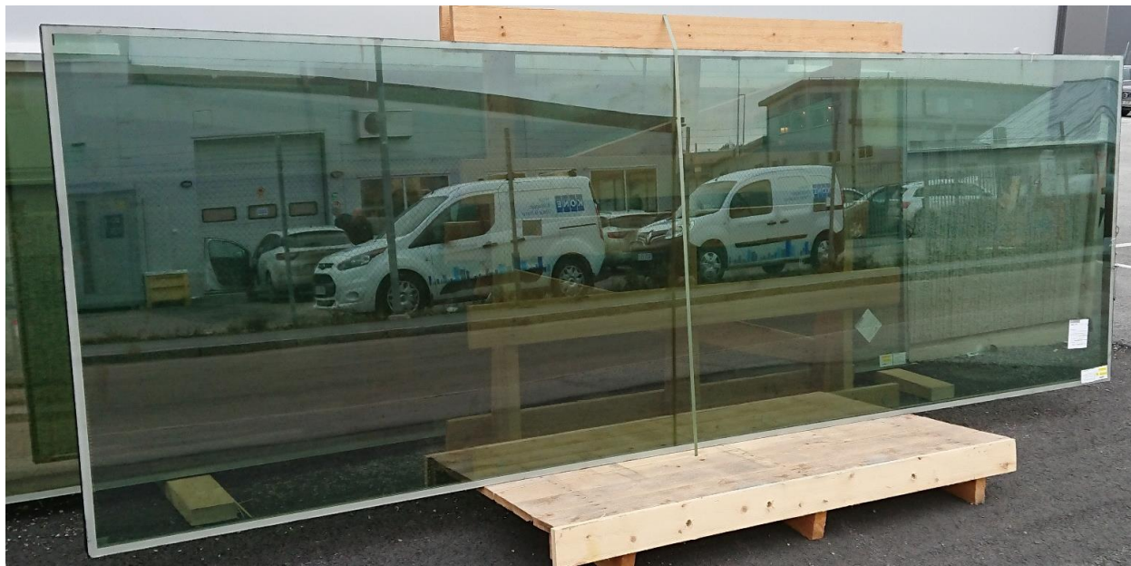
large area electrochromic demo (IGU 4.42 m 2 )
