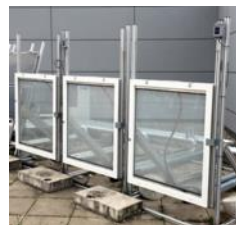
PS+ semi-transparent microfluidic heat storage system prototypes
