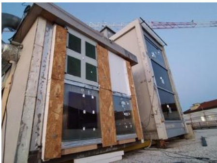
POWERSKIN PLUS outdoor test cells
