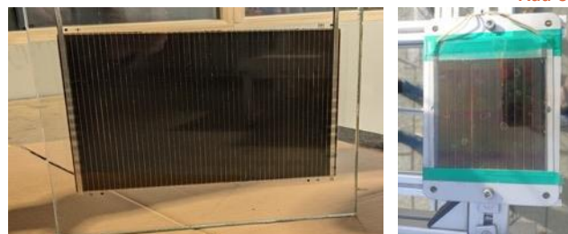
PS+ Opaque flexible perovskite PV prototype
