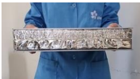
PS+ VIP insulation prototype
