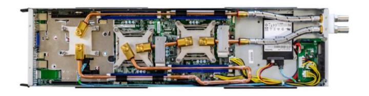
Server blade, with direct-on-chip cooling capable of generating water of up to 60°C – sufficient for heating applications directly or boosted with a heat pump.
