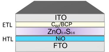
**Zn(O,S):** layers with suitable composition (Eg 2.8 eV) are compact and without holes. However: need to increase grain size
