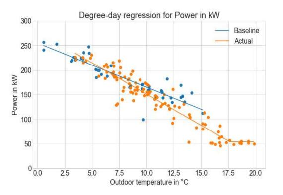
Preliminary results suggest less network power consumption, most likely due to reduction in distribution heat losses.
