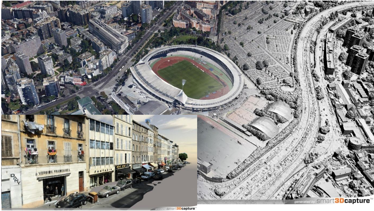
Figure 31: Example of 3D automatic capture using Smart3DCapture technology from ACute3D (Credentials: InterAtlas, Visuel3D, and Acute3D).
