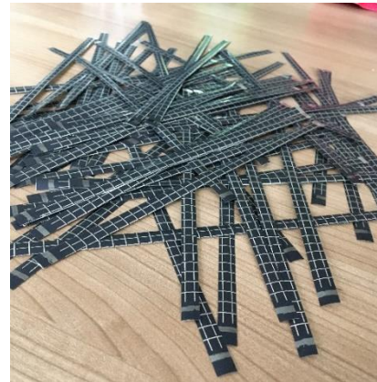
Customized solar module stripe fabrication
