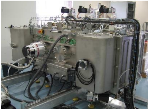
Reactive sputtering process
