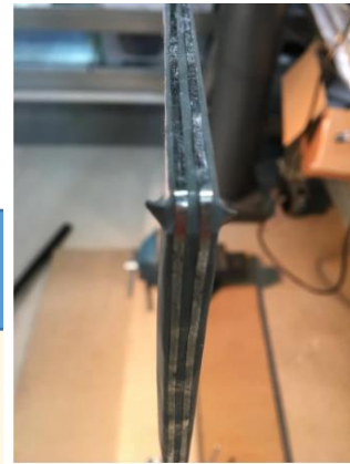
Solar module coupling to laminate
