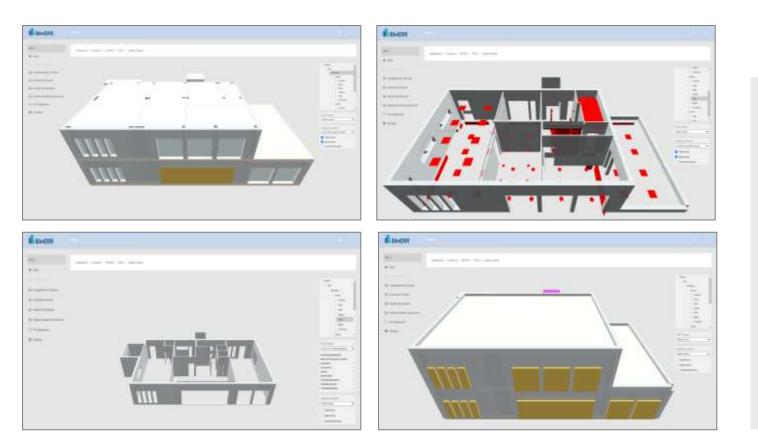
**BIM Platform**: A toolset that optimises and checks the completeness & correctness of the BIM model
