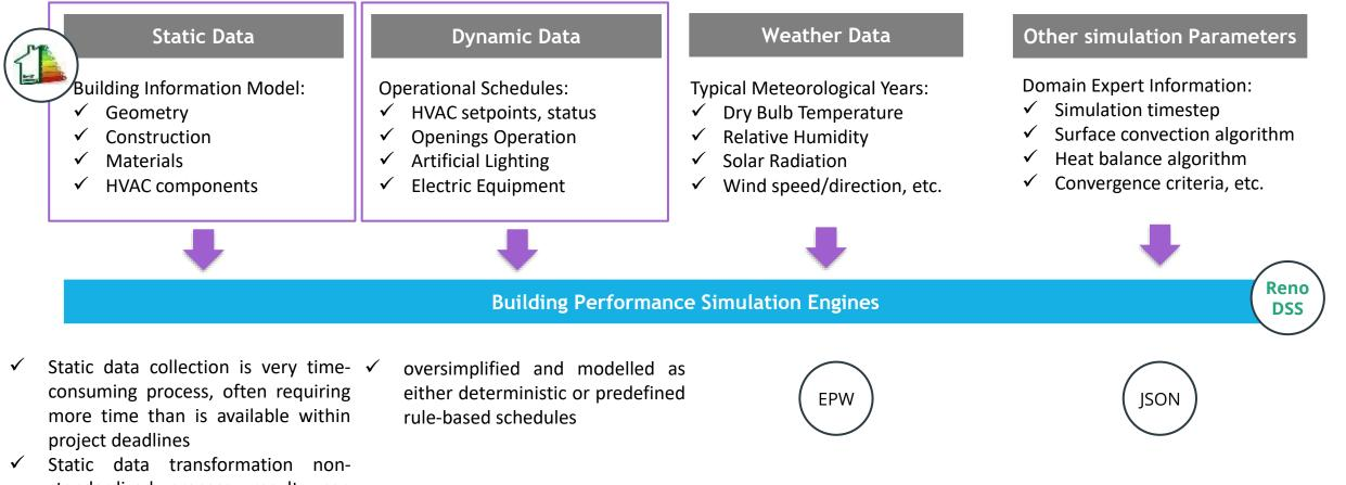
Static data transformation nonstandardized process; results can significantly vary from one modeller to another
