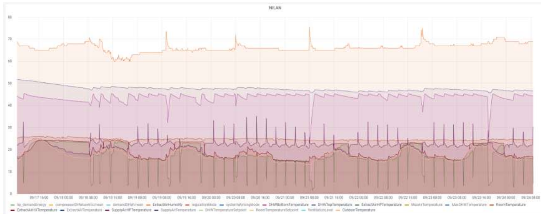
Data from the Nilan equipment and the indoor conditions of the house
