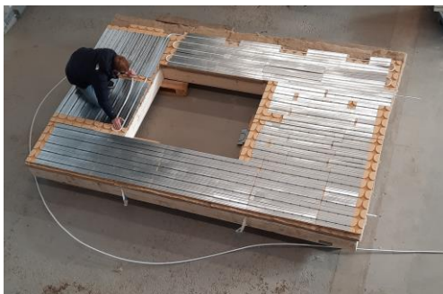
Construction of the Heating layer on a Prototype
