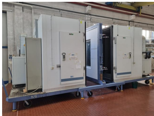
Guarded hot box for Thermal Transmittance / Thermal Resistance of opaque components and glazing system
